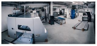
3D printers for sandmolds and cores
