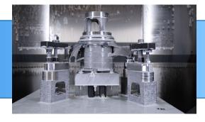
Stator Housing for Electric Motor including synthetic core
